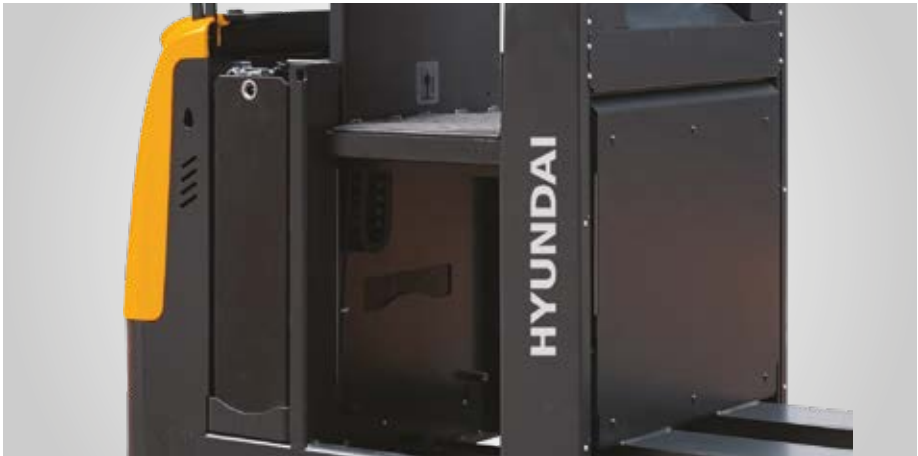
The coasting button on both sides of the order picker enables the operator to move the order picker forward or backward and lift the forks while walking alongside. This eliminates the need for frequent entry and exit, significantly improving picking efficiency and operational safety.
