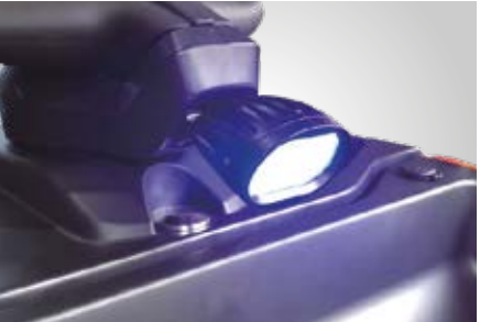
The standard front blue light is automatically activated when the order picker is driving forward and also turns simultaneously with the handle during steering, thereby enhancing operational safety.
