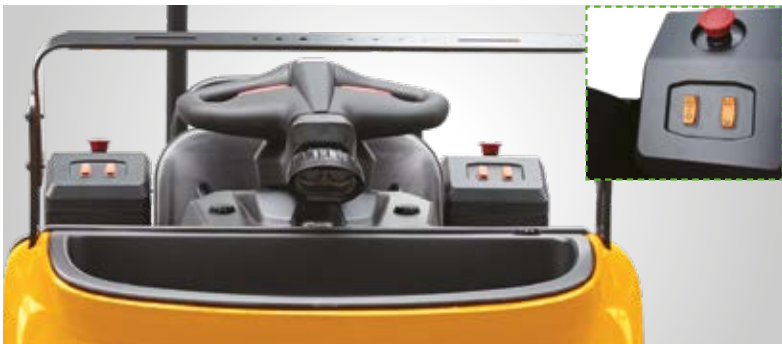
The coasting button on both sides of the order picker enables the operator to move the order picker forward or backward and lift the forks while walking alongside. This eliminates the need for frequent entry and exit, significantly improving picking efficiency and operational safety.
